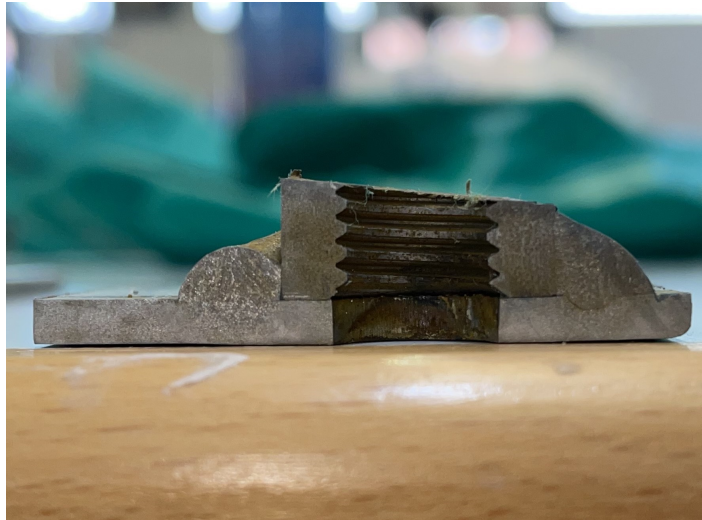
(a) Etched Upper Module Weld
